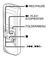
When "REC-OP" in the menu is set to "ADD," you can add a recording to the message being played back. The added recording will be placed after the current message, and will be counted as a part of the message. During playback of Message 3
